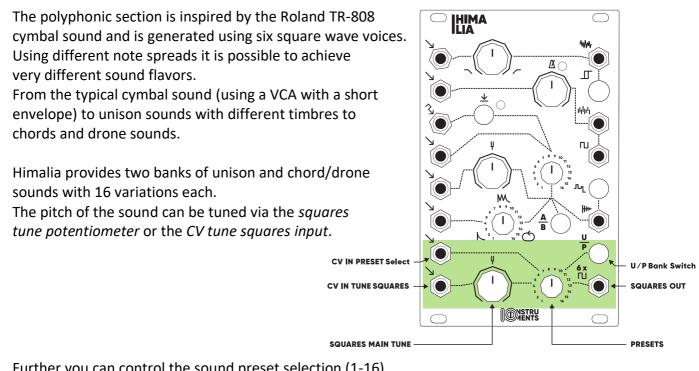
Further you can control the sound preset selection (1-16) by using the *preset potentiometer* or the *CV preset input*. Banks can be switched from unison to chord presets and vice versa via the *U / P bank button*. (disengaged: unison; engaged: chord sounds)
